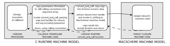
Figure 9. Control flow of a callback (solid lines for main invocation; dashed for return)
