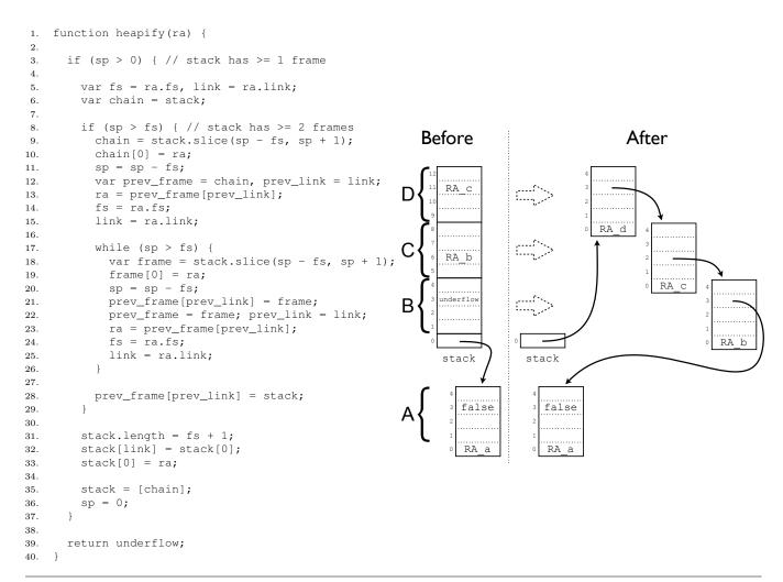
Figure 7. Continuation heapification algorithm and example. Before heapification, continuation frames B, C and D are on the stack. After heapification with the call heapify(RA\_d), where RA\_d is the return address back to the function that created frame D, all frames are in the heap and explicitly linked using the frame slot normally containing the return address.
